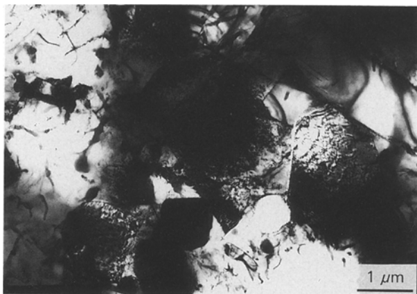
Figure 10 Typical grain morphologies of the \text{Si}_3\text{N}_{4w}/\text{Al-Mg-Si} aluminium composites after extrusion at a high reduction ratio of 100:1.
